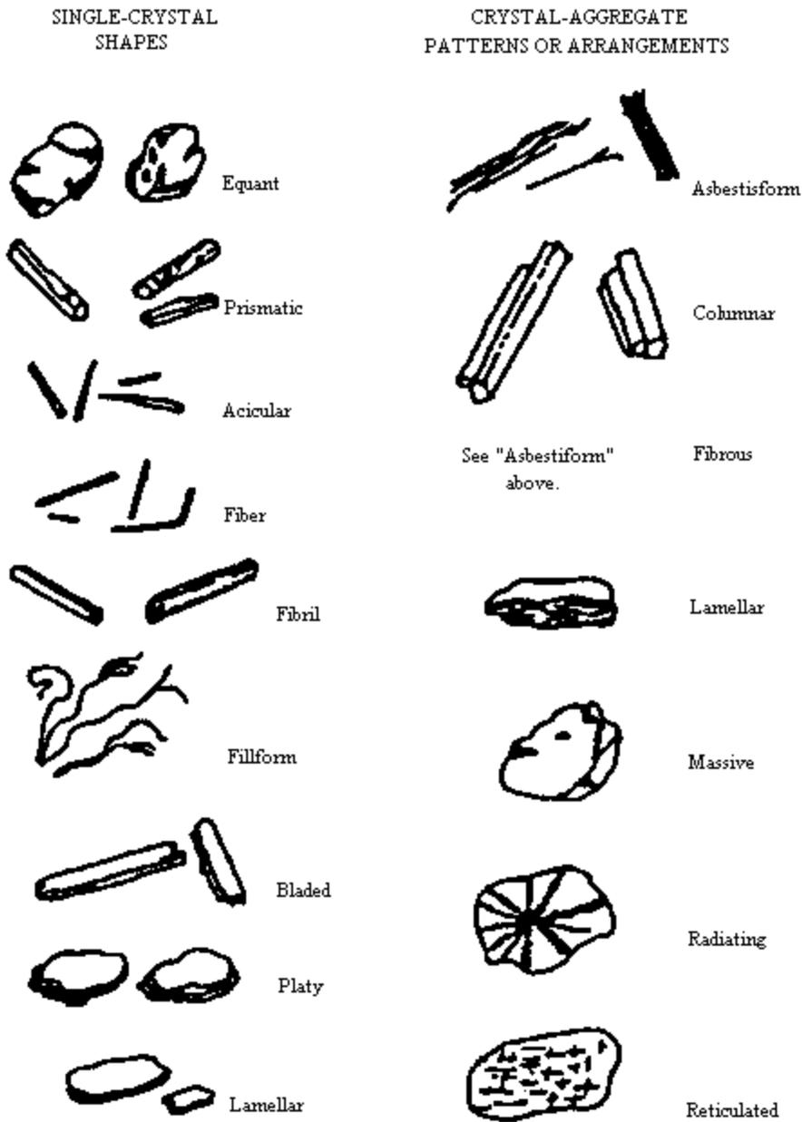
Figure 1. Particle definitions showing mineral growth habits.
